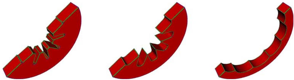
Fig. 12 Simulation of uniform burning of section of star grain of solid rocket using face-offsetting and mesh repair. Green curves indicate ridges in evolving geometry
