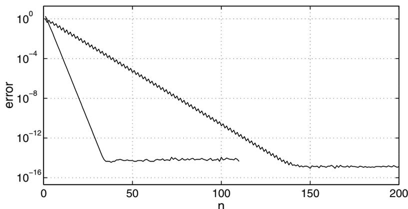
**Fig. 6.1** Convergence of the error (6.1) in polynomial interpolation of two smooth functions  $f$  in Chebyshev points of the second kind in  $[-1, 1]$ . The lower curve corresponds to  $f(x) = \exp(x)/\cos(x)$ , and the upper curve to  $f(x) = (1+16x^2)^{-1}$ . In both cases we observe steady convergence down to the level of rounding errors. The wiggles in the second function arise from the missing central node for odd  $n$ .
