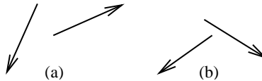
Fig. 2. For two segments to be eligible to be adjacent each should have at least one endpoint on the left side of the other. (a). Segments are eligible to be adjacent; (b). Segments are ineligible to be adjacent.
